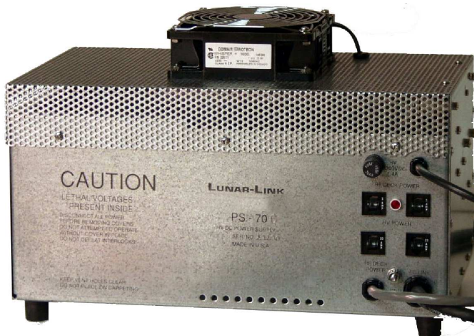
Optional external cooling fan mounted to the power supply cover.
